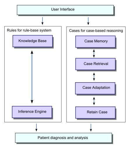
Figure 4 Hybrid expert system architecture
