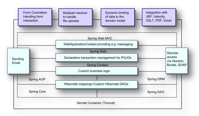
Figure 6 Typical full-fledged Spring web application
