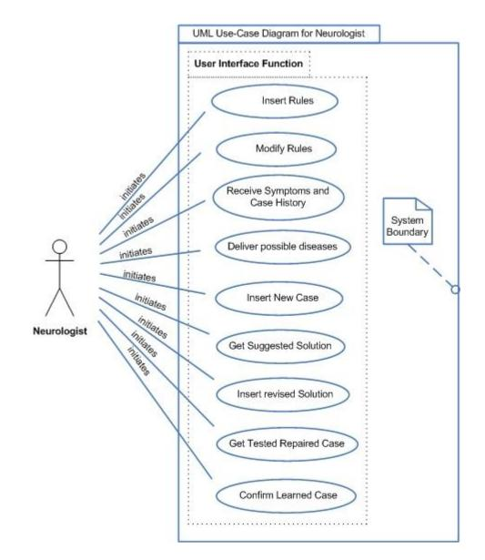
Figure 8 UML USE case diagram for a neurologist
